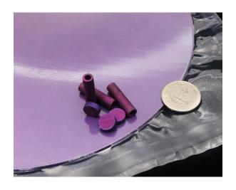
Lanthanum Hexaboride (LaB<sub>6</sub>) Rod/Tube/Plate Crucible/Electrode
